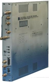
The WJ-8635 is a fully synthesized, general-purpose HF/ VHF/UHF receiver tunable from 20 to 1000 MHz, and extendable down to 0.5 MHz or up to 2.4 GHz.
